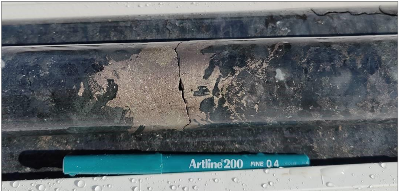
Figure 5. Coarse sulphide with visible pentlandite at 414m.
